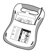
The pad package can then be stored in the pad storage slot in the back of the *DDU-120* AED. After connecting the pads connector to the unit, push the pad package, with the pictures on the package facing up and out, rounded end first, into the pad holder compartment on the back of the AED. When the pad pack is fully inserted, press the pad cable into the groove in the back of the unit to hold it in place and tuck any excess cable behind the pad package.
