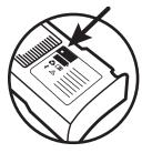
The battery pack's Active Status Indicator ("ASI") is located on the label face of the battery pack and is used to indicate battery pack status. A periodically blinking green LED indicates that the battery pack status is OK and the battery pack is ready for use. Absence of a blinking green LED indicates a battery pack problem or a depleted or missing 9V battery. Refer to the "Checking DDU-120 AED Status" section for information on battery pack LED indications.
